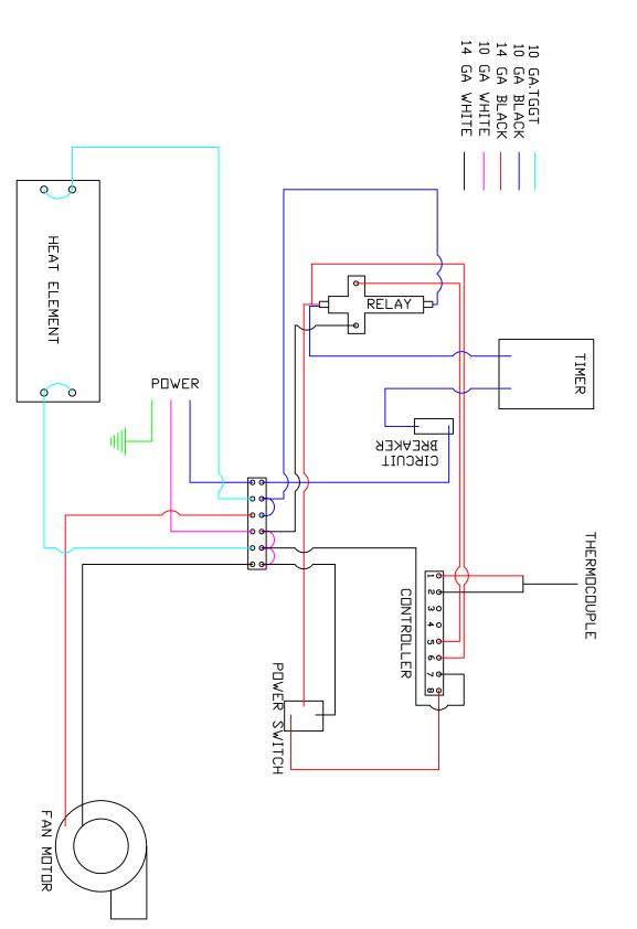
H5 WIRING DIAGRAM CHANGE FROM MERCURY RELAY RELAY
